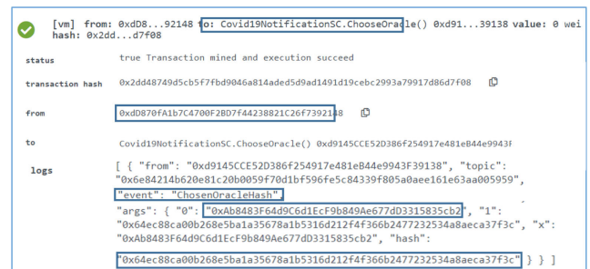
FIGURE 9. Logs showing a successful announcement of the chosen list hash and the winning registered oracle.
