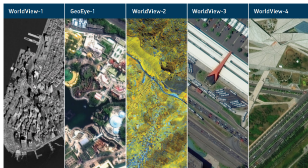
FIGURE 1. Multi-domain images provided by the Digital Globe 3 satellites [5]. The images lie on different domains according to operational altitude, spectral characteristics, and resolutions.
