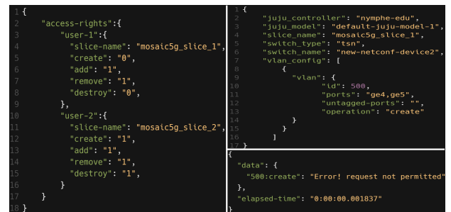
FIGURE 10. (left) Slice access rights, (top right) VLAN creation, and (bottom right) JOX NBI output for access violation.
