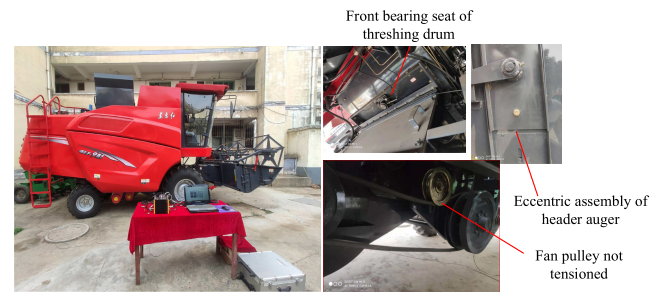
FIGURE 2. Positions of the measuring points on the test harvester.
