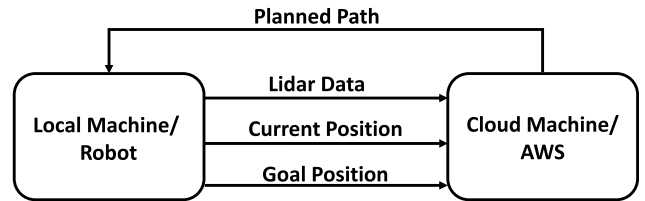
FIGURE 5. Robot-AWS communication framework. The robot forwards LiDAR data (obstacles) and the current and goal positions to AWS. AWS calculates and forwards the shortest path between those positions to the robot.
