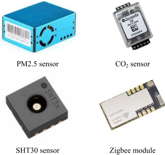
FIGURE 2. Sensors and wireless module used in IAQD.
