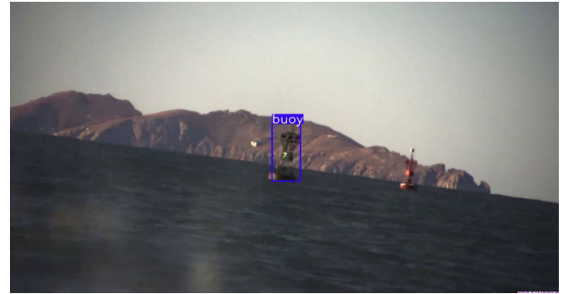
FIGURE 7. Effect of the first-frame object extraction algorithm In the case of multiple buoys (complex background).
