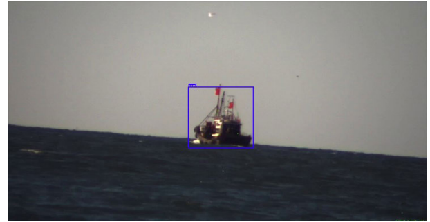
FIGURE 14. First-frame object extraction algorithm for ship extraction.
