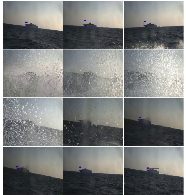
FIGURE 21. Object tracking effect in the case of seawater blocking the lens.
