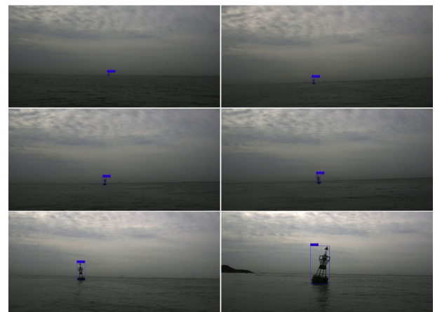
FIGURE 18. Object tracking effect in cloudy weather.
