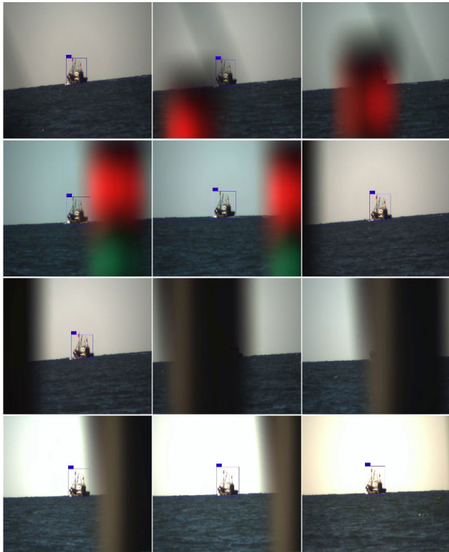
FIGURE 20. Object tracking effect in the case of mast blocking the lens.
