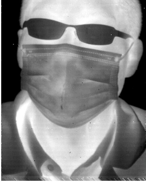
FIGURE 5. Image taken by the MOCVD-grown LWIR T2SL FPA camera with an integration time of 1.9 ms.
