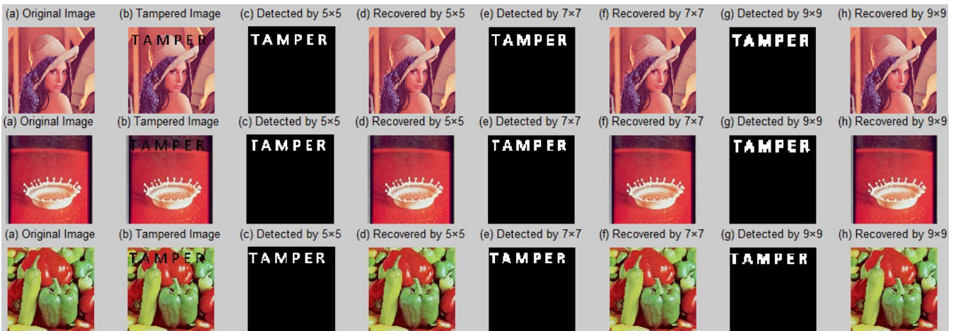
FIGURE 21. (a) Original Color Image, (b) Tampered Image, (c and d) Detected and recovered image by 5 \times 5 , (e and f) Detected and recovered image by 7 \times 7 , (g and h) Detected and recovered image by 9 \times 9 .
