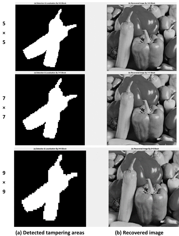
FIGURE 16. Detecting and Recovering tampered image by 5 × 5, 7 × 7 and 9 × 9 Blocks respectively from top to bottom shows more precision in block size 5 × 5.
