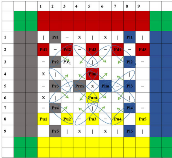
FIGURE 13. Recovery of a tampered block using backup recovery when the first recovery data are lost for a block size of 9 × 9.
