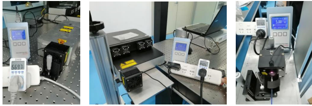
(a) Electric power test. (b) Laser power test. (c) Laser power test after beam expansion.
