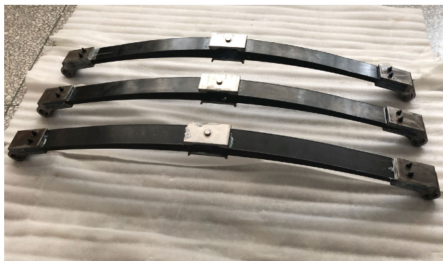
FIGURE 6. Samples of the composite leaf spring.
