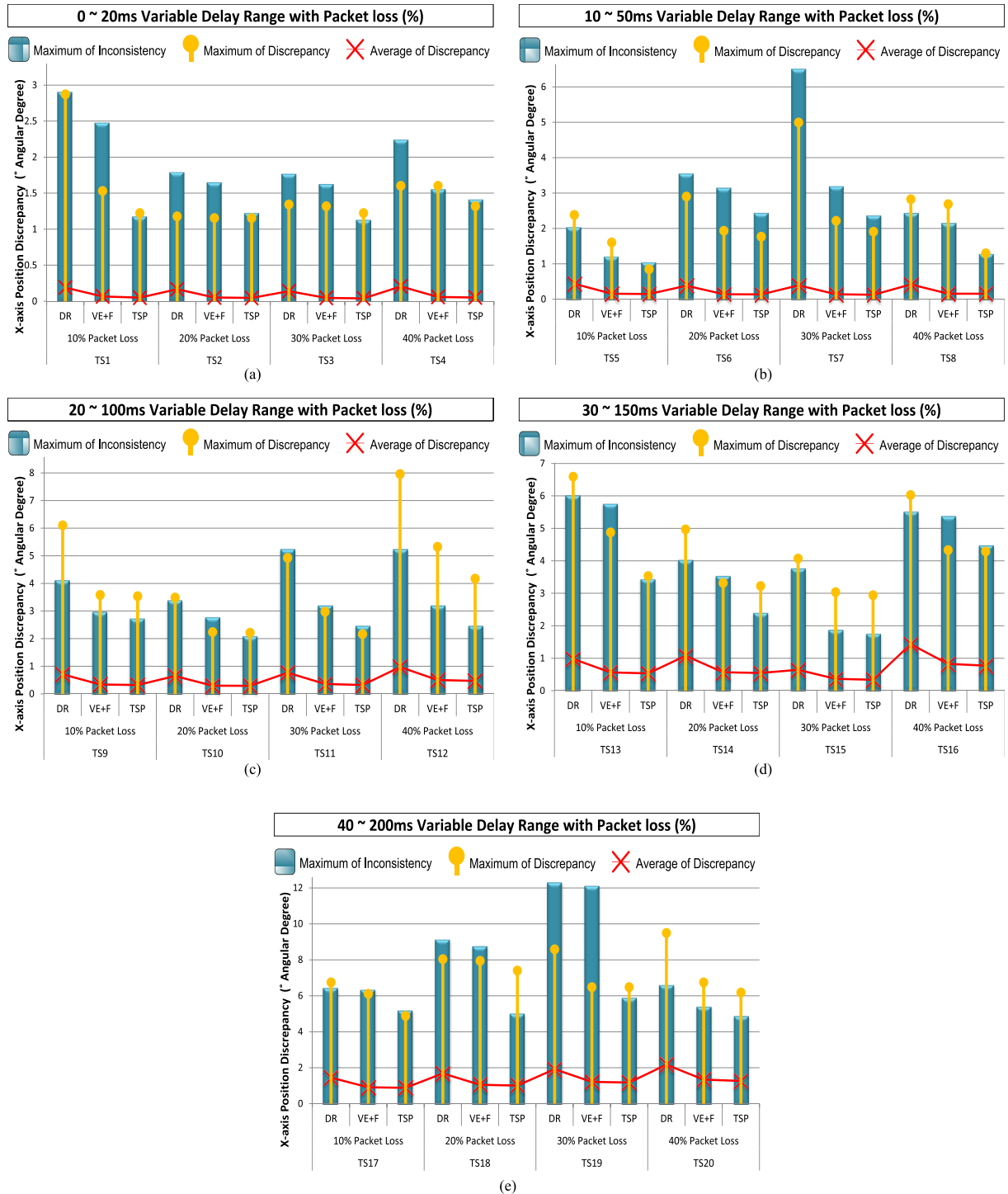
FIGURE 9. Comparison of Prediction Techniques with (a) up to 20ms variable delay with 10% packet loss in TS1, 20% in TS2, 30% in TS3, and 40% in TS4; (b) 10ms to 50ms variable delay with 10% packet loss in TS5, 20% in TS6, 30% in TS7, and 40% in TS8; (c) 20ms to 100ms variable delay with 10% packet loss in TS9, 20% in TS10, 30% in TS11, and 40% in TS12; (d) 30ms to 150ms variable delay with 10% packet loss in TS13, 20% in TS14, 30% in TS15, and 40% in TS16; (e) 40ms to 200ms variable delay with 10% packet loss in TS17, 20% in TS18, 30% in TS19, and 40% in TS20.
