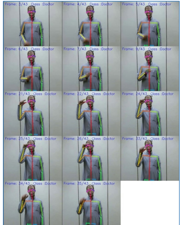
FIGURE 6. Hand skeleton generation errors, right hand fully/partially blurred (Dynamic Sign)— finger joints not identified.
