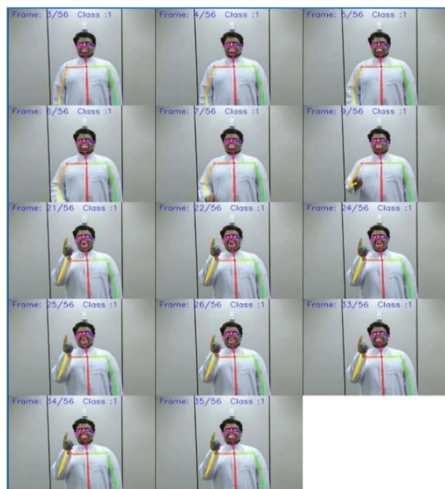
FIGURE 4. Example of the OPL output on the ArSL dataset, static sign—joints correctly identified.
