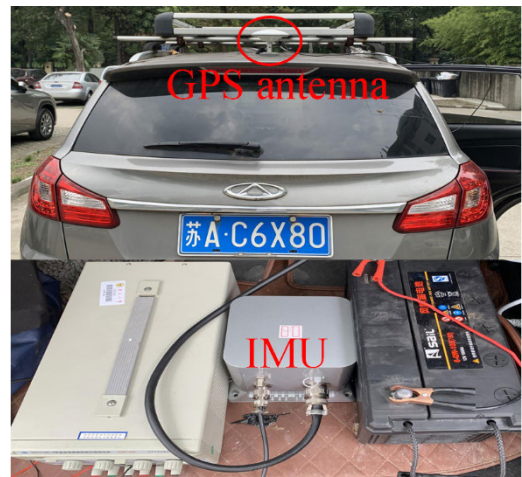
FIGURE 13. Equipment installation diagram in field test.
