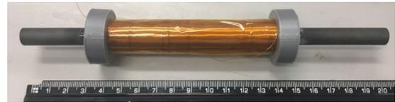
FIGURE 6. The fabricated solenoid energy harvester.
