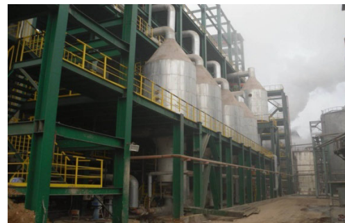
FIGURE 13. The evaporation process of the alumina production in an aluminum metallurgical plant.
