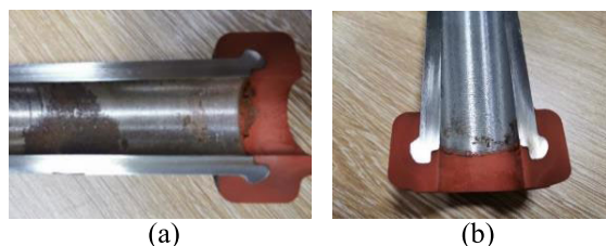
FIGURE 5. Dissection test results of the end fittings: (a) Seriously erosion, (b) Slightly erosion.
