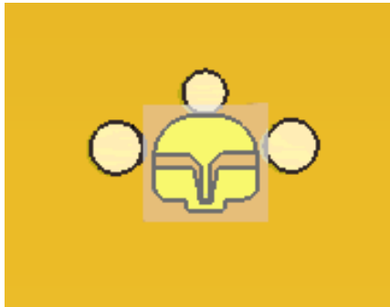
FIGURE 13. The layer model with the fat tunnels on the sides of the antenna substrate.
