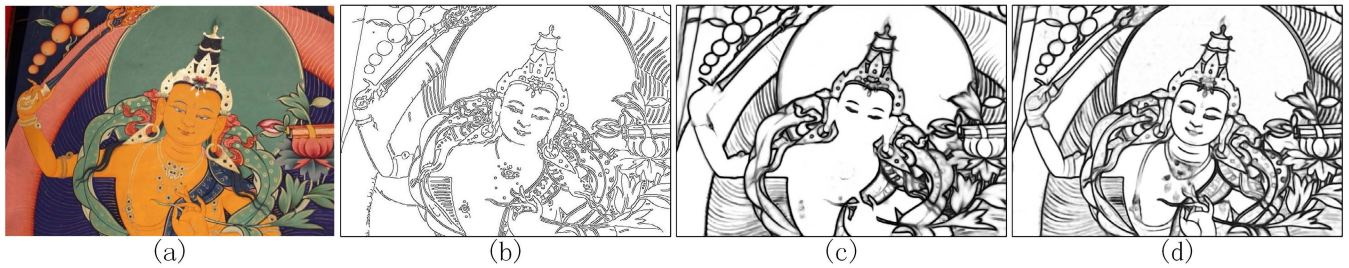
FIGURE 1. The proposed RITE-Net achieved the best edge-map with richer image semantics and more edge details (Fig.1(d)). The existing learning-based methods failed to generate vital edge details (eg: no face, hand and breast details in Fig.1(c)) while traditional non-learning method such as Canny tends to either generate fake edges or lacks important edges because of the absence of high-level image semantics (Fig.1(b)). Fig.1(a)) is a Thangka mural.
