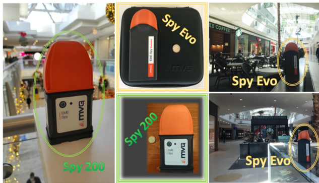
FIGURE 3. EME SPY Evolution and EME SPY200 personal dosimeters used for the measurement campaign within the shopping malls.
