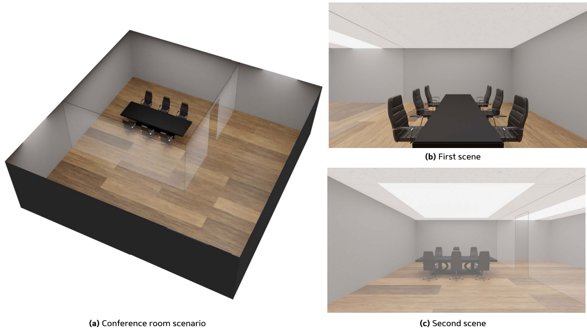
FIGURE 23. (a) the bird view of the conference room scenario; (b) and (c) the scenes under study. The 10\text{m} \times 10\text{m} indoor space contain a 6\text{m} \times 6\text{m} conference room in glass. the indoor space walls are made from layered drywall, the ceiling is made from ceiling board and the floor is made from floorboard. The conference room chairs and tables are made from wood.
