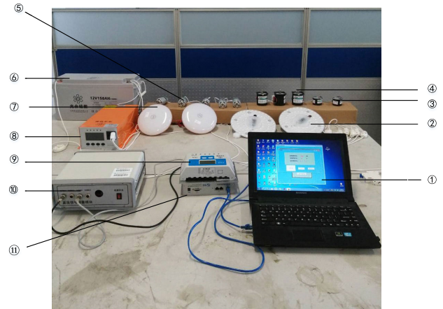
FIGURE 10. Photovoltaic energy metering device experimental platform diagram: ① computer; ② 36 w AC bulb; ③ 10 w AC motor; ④ 28 w AC motor; ⑤ 20.4 w DC motor; ⑥ battery; ⑦ 50 w DC bulb; ⑧ inverter; ⑨ controller; ⑩ signal measurement module; AD conversion module.
