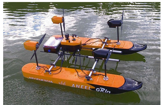
FIGURE 1. Real view of the developed catamaran.
