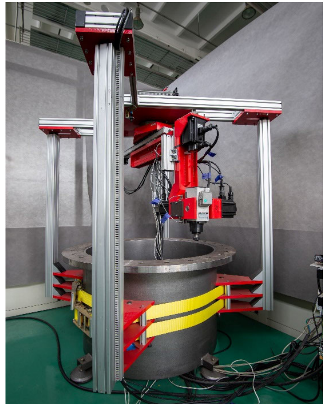
FIGURE 7. Constructed prototype of portable machine tool.
