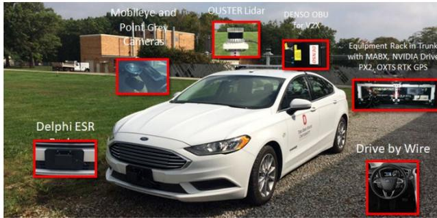
**FIGURE 5.** Ford Fusion automated experimental vehicle of the Automated Driving Lab at the Ohio State University. This drive-by-wire vehicle is equipped with sensors as well as data processing and control units to achieve autonomous driving. Its model parameters were validated through vehicle dynamics testing, to represent the vehicle inside the simulations with high accuracy and design realistic controllers.
