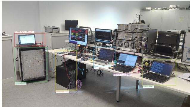
FIGURE 4. The Emulradio4Rail platform with one LTE bearer emulated by OAI and FPGA based channel emulator in the IKERLAN laboratory.
