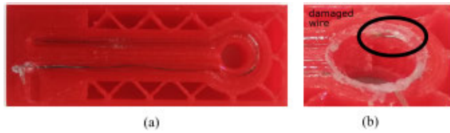
FIGURE 16. Method for contacting embedded wires through displacement with a conical shaped insert (a) printed structure with a wire path forming a ring, in which the threaded insert is pressed in (b) damaged wire after removing the insert to inspect the contact geometry.
