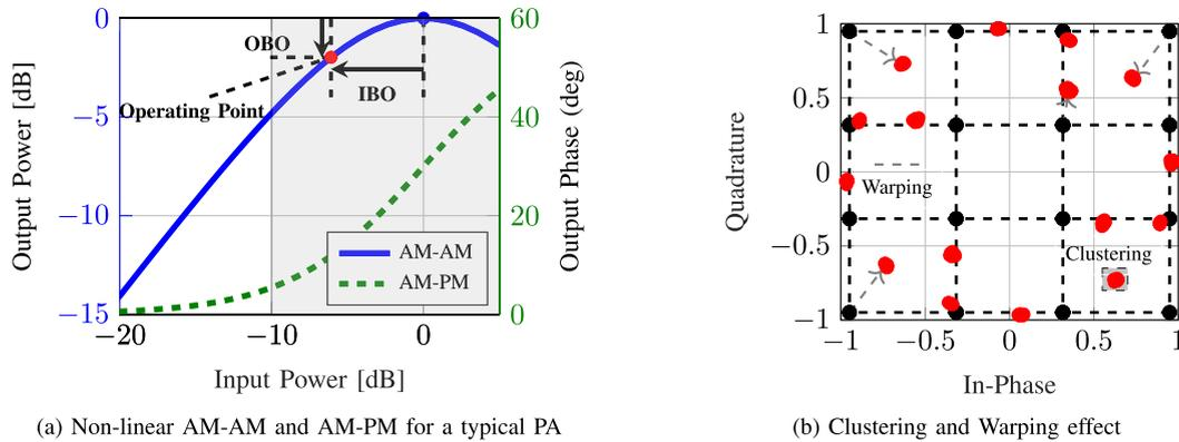
FIGURE 1. HPA and the associated non-linear characteristics.
