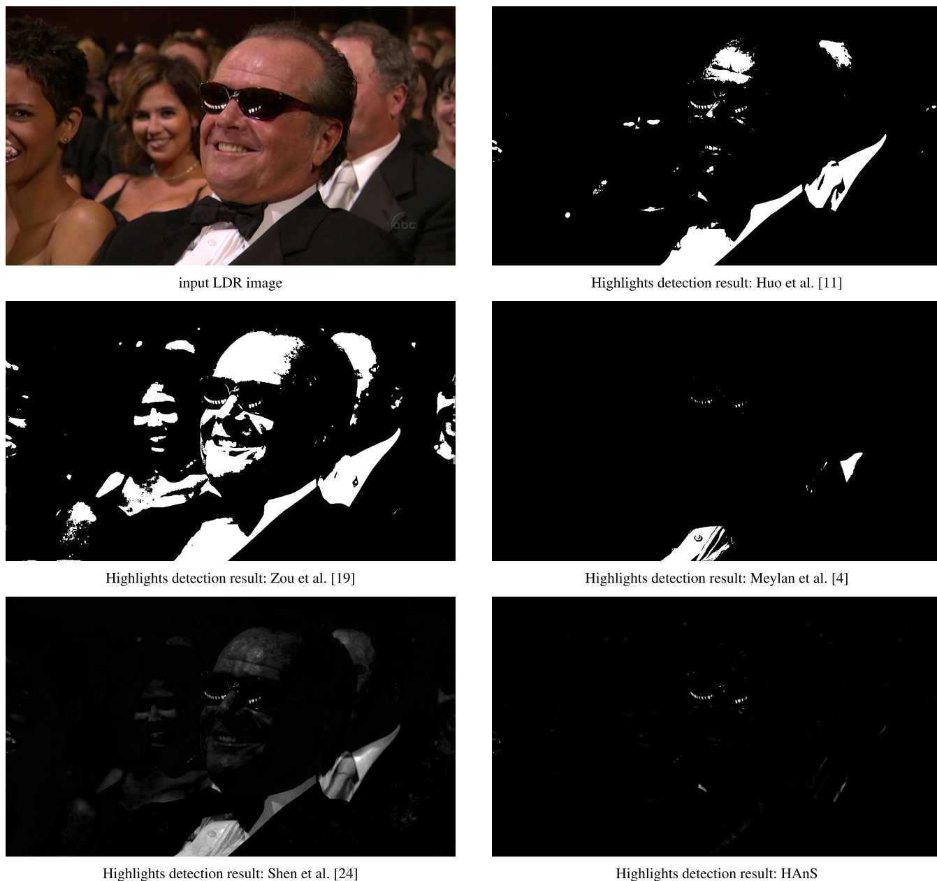
FIGURE 11. Results from highlights detection algorithms on Example 2. Note that HAnS produces the least amount of incorrect detections (areas that belong to light reflections from bright diffuse surfaces).
