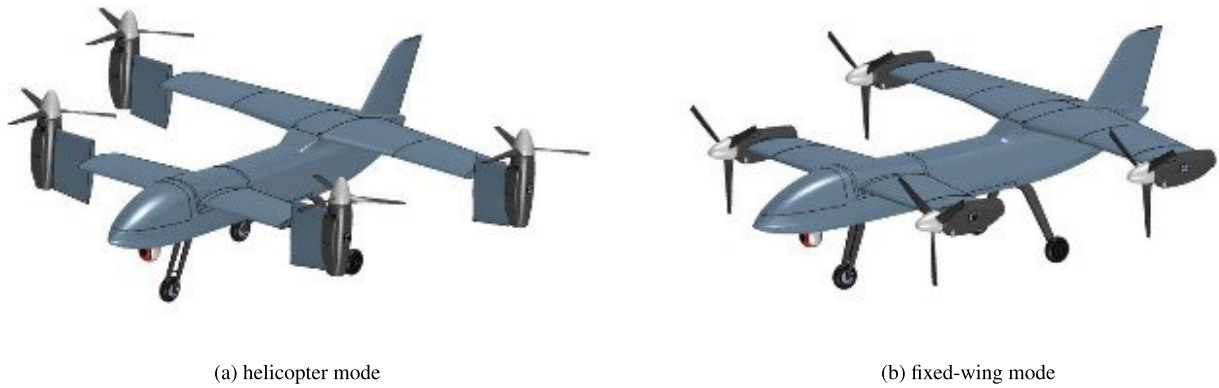
FIGURE 1. 3D model of quad tilt rotor with partial tilt wing.
