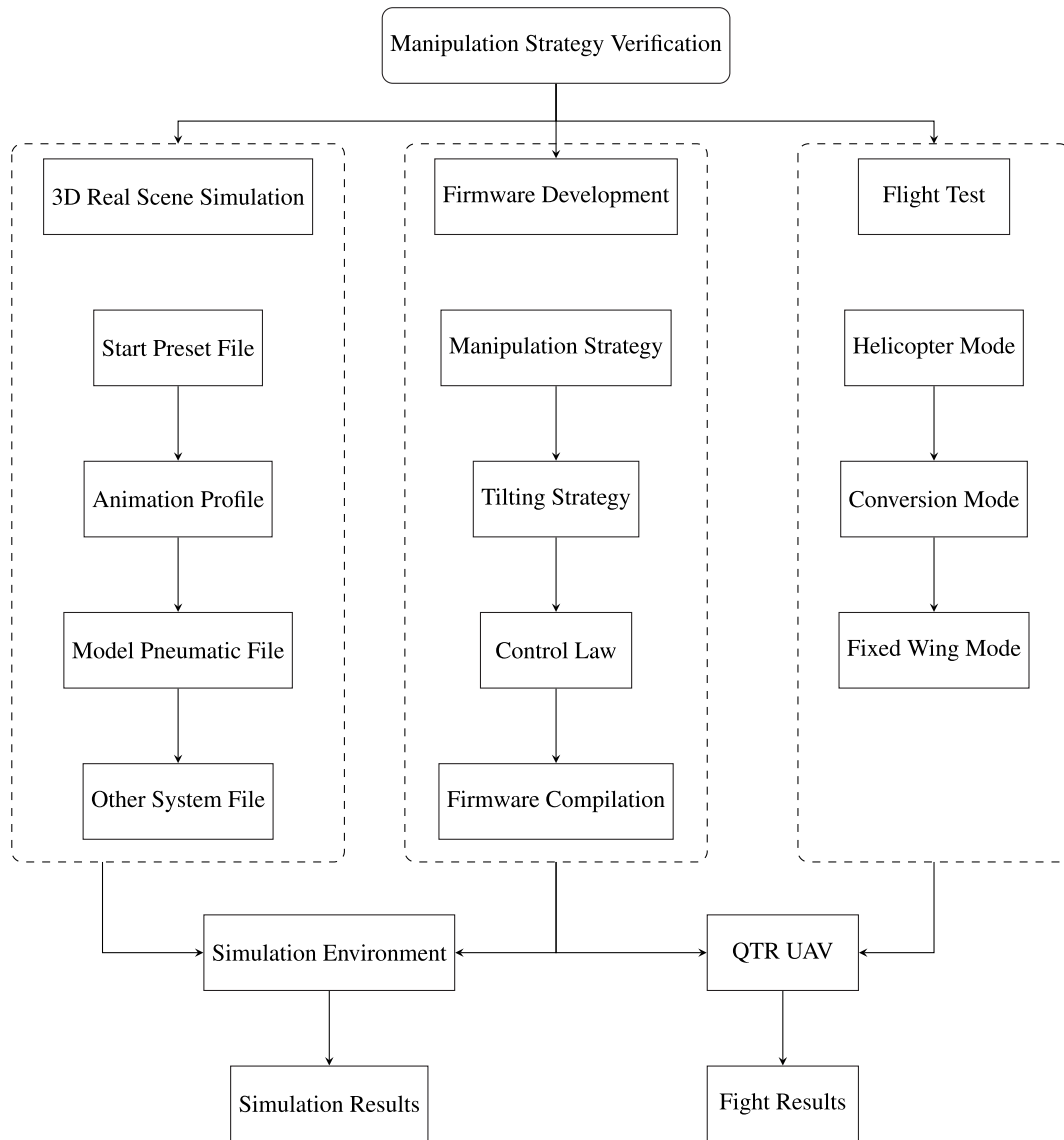
FIGURE 14. Flight test verification process.
