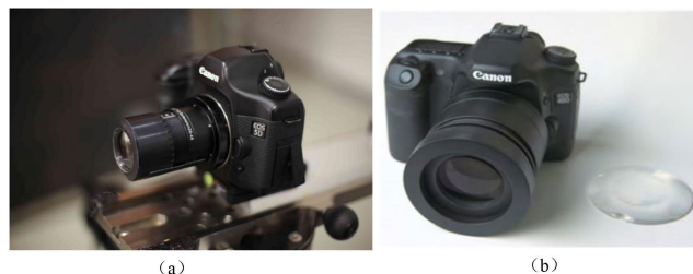
FIGURE 1. (a) Single-lens camera made by Schuler [5] with one lens. (b) Single-lens camera made by Heide et al. [6] with one lens.
