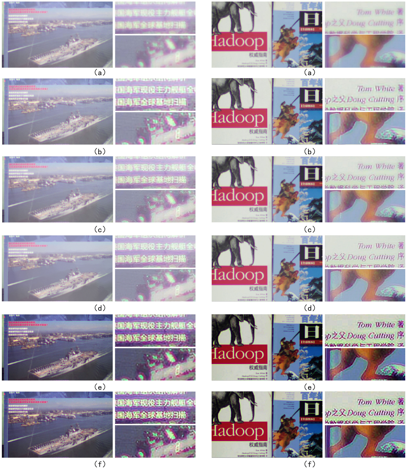
FIGURE 17. Image restoration results of simple-lens camera with two lenses in Figure 1 (b). (a) Blur image pictured by simple-lens camera with two lenses; (b) Image restoration result with PSF estimation of Xu [22]; (c) Image restoration result with PSF estimation of Dong [24]; (d) Image restoration result with PSF estimation of Yan [25]; (e) Image restoration result with PSF estimation of the proposed method without NSAS model; (f) Image restoration result with PSF estimation of the proposed method using NSAS model.
