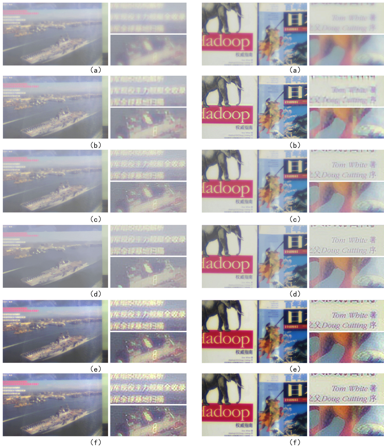
FIGURE 16. Image restoration results of simple-lens camera with one lens in Figure 1 (a). (a) Blur image pictured by simple-lens camera with one lens; (b) Image restoration result with PSF estimation of Xu [22]; (c) Image restoration result with PSF estimation of Dong [24]; (d) Image restoration result with PSF estimation of Yan [25]; (e) Image restoration result with PSF estimation of the proposed method without NSAS model; (f) Image restoration result with PSF estimation of the proposed method using NSAS model.
