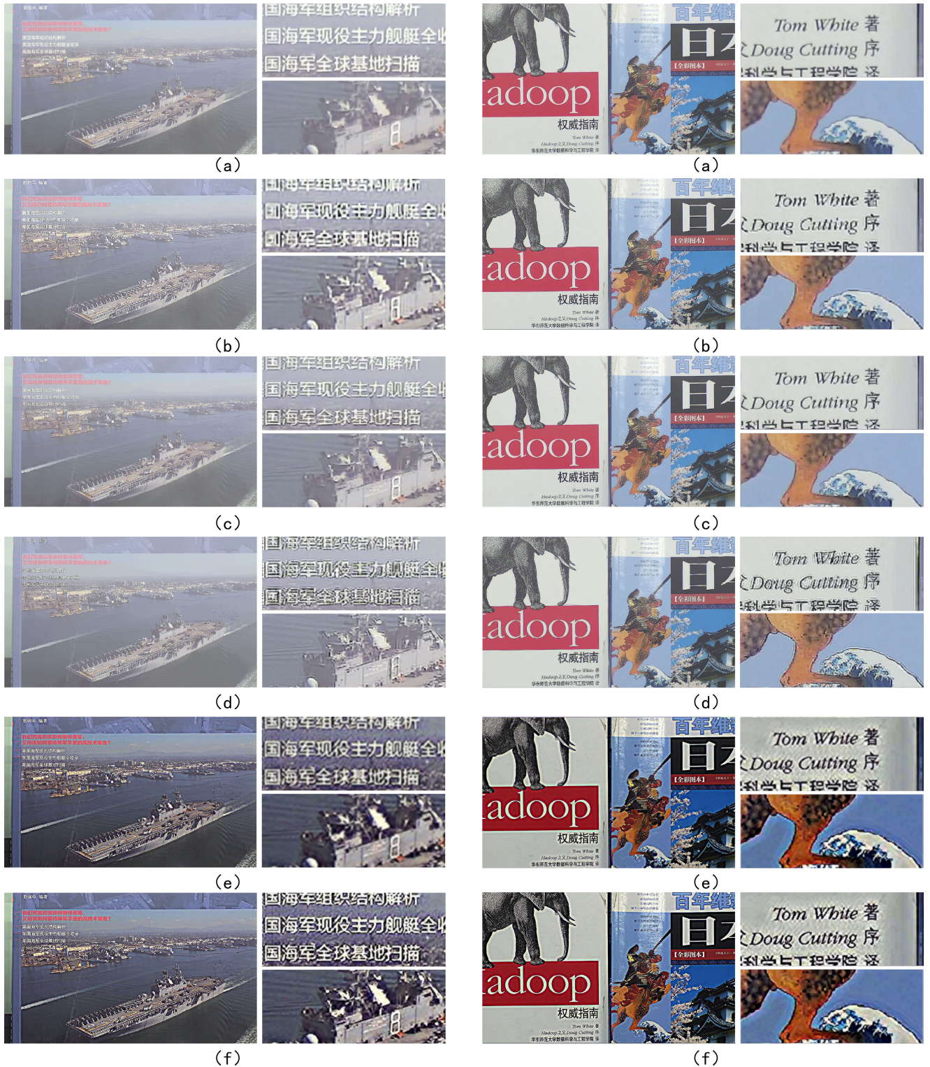
FIGURE 18. Image restoration results of simple-lens camera with three lenses in Figure 1 (c). (a) Blur image pictured by simple-lens camera with three lenses; (b) Image restoration result with PSF estimation of Xu [22]; (c) Image restoration result with PSF estimation of Dong [24]; (d) Image restoration result with PSF estimation of Yan [25]; (e) Image restoration result with PSF estimation of the proposed method without NSAS model; (f) Image restoration result with PSF estimation of the proposed method using NSAS model.
