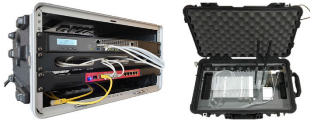
FIGURE 6. Portable PPDRone mobile system facility deployment (left) and PPDR IoT toolkit for field use (right).
