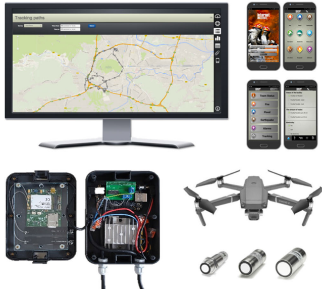
FIGURE 7. PPDR applications available in the PPDRone facility – an intervention monitoring dashboard (top left) with field triage and tracking mobile application (top right); a sensor gateway (bottom left), and a drone and ultrasonic water level sensors (bottom right).
