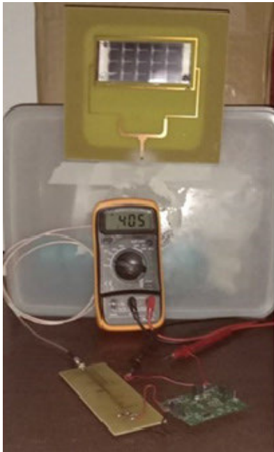
FIGURE 25. The measurement of the hybrid harvester in a dark or night environment.
