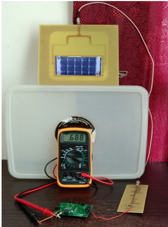
FIGURE 23. Evaluation of Hybrid harvester using the BQ-25504 power management module (PMM).
