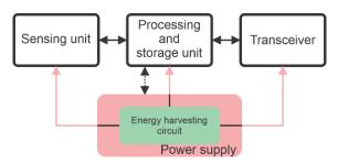
(a). Wireless sensor (IoT device) with energy harvesting architectures: Harvest-Use. Adapted from [32].
