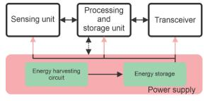
(b). Wireless sensor (IoT device) with energy harvesting architectures: Harvest-Store-Use. Adapted from [32].
