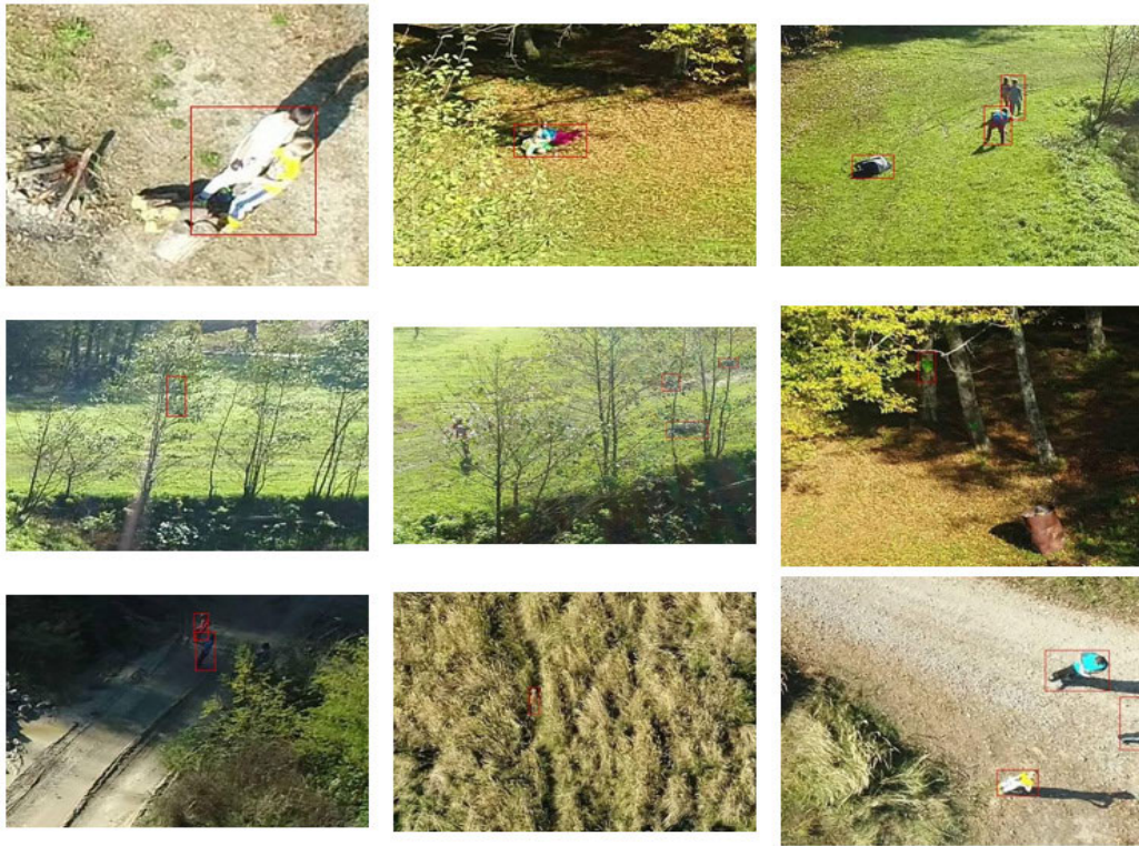
FIGURE 12. Miss detections of the YOLOv4 (SARD) model (cropped images to make it easier to notice the persons in the image): two people are standing very close to each other or overlapping (first row); darker parts of vegetation detected as a person (second row); shadows detected as persons (third row).
