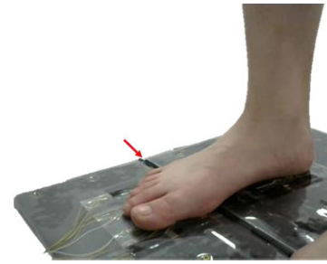
FIGURE 11. Position of the transverse arch (red arrow), which is the turning point when the platform rises.
