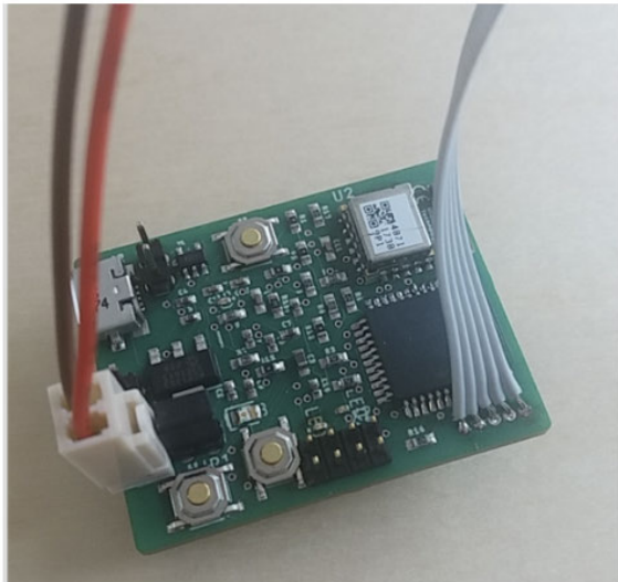
FIGURE 9. Prototype V2 (Bluetooth): integrated final electronic board.
