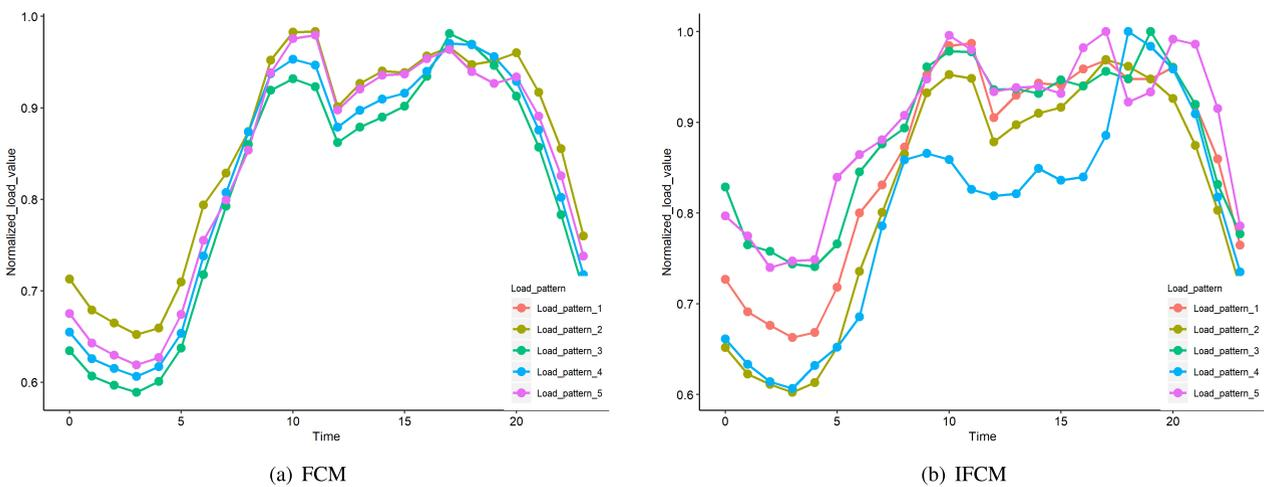
**FIGURE 6.** Load patterns clustered by the FCM and IFCM clustering algorithms on D\_China data set.
