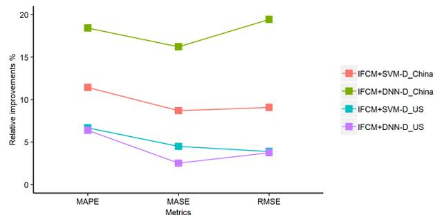
FIGURE 13. The percentages of the relative improvements by combining IFCM with SVM and DNN on the two data sets.
