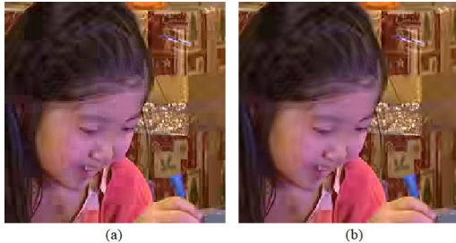
FIGURE 2. Example of using deblocking filter in BlowingBubbles frame, encoded at QP37: (a) DB disabled, (b) DB enabled.
