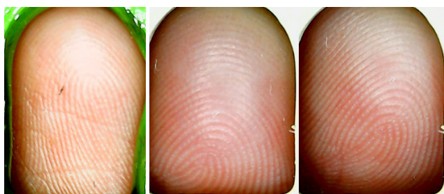
FIGURE 18. Samples of infant fingerprints which displayed specular reflection under white LED ring illumination.
