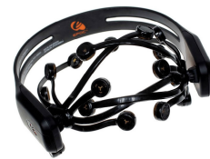
FIGURE 6. Emotiv Epoc headset has a gyroscopic sensor and 14 EEG electrodes distributed in the right and left hemispheres of the brain, a sample rate of 128 Hz and wireless EEG system.
