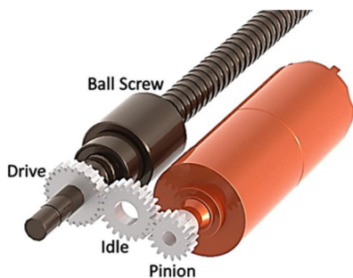
FIGURE 1. Schematic of BS linear actuation drive.
