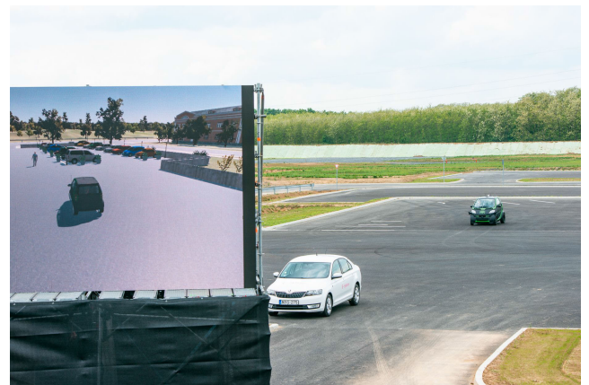
FIGURE 8. The proof of concept demonstration of the mixed-reality based SciL concept at ZalaZONE 20/05/2019. The green Smart (VUT) moves fully autonomously in a valet parking scenario; the white Skoda is simply parking. The big screen on the left side displays the digital twin of ZalaZONE and the real-time movement of the VUT in it. The parking lot is empty in reality, while it is occupied by virtual vehicles in its digital representation. A virtual pedestrian is just stepping out from behind one of the virtual cars, making the VUT stop in reality as well. (video available: https://youtu.be/Ue3W7cjUtf8 ).
