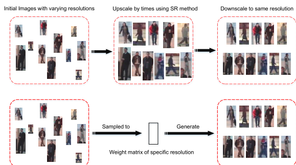
FIGURE 2. Illustration of mechanism differences between the typical SR methods and ours in cross-resolution person re-id dataset, CAVIAR. Compared to the general SR methods, we generate the images of same resolution in one step using a weight matrix of specific resolution.
