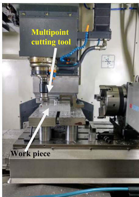
FIGURE 6. Machining of the square ring force transducer.
