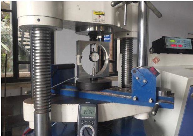
FIGURE 17. Verification of uniaxial testing machine.
