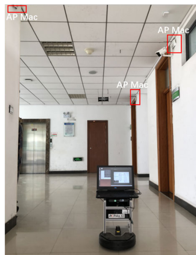
FIGURE 3. Testing of the hardware platform in an indoor scene with many AP Macs mounted on the wall.
