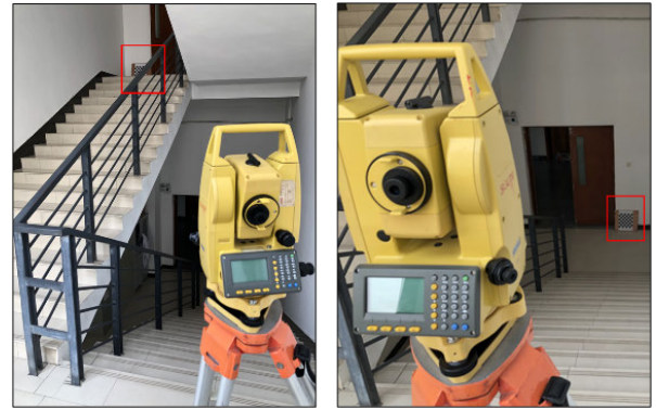
FIGURE 6. Hi-Target ZTS-121 Total Station is used as a building control point to unify the maps of various floors (the red boxes in the images are landmarks for more precise surveying).
