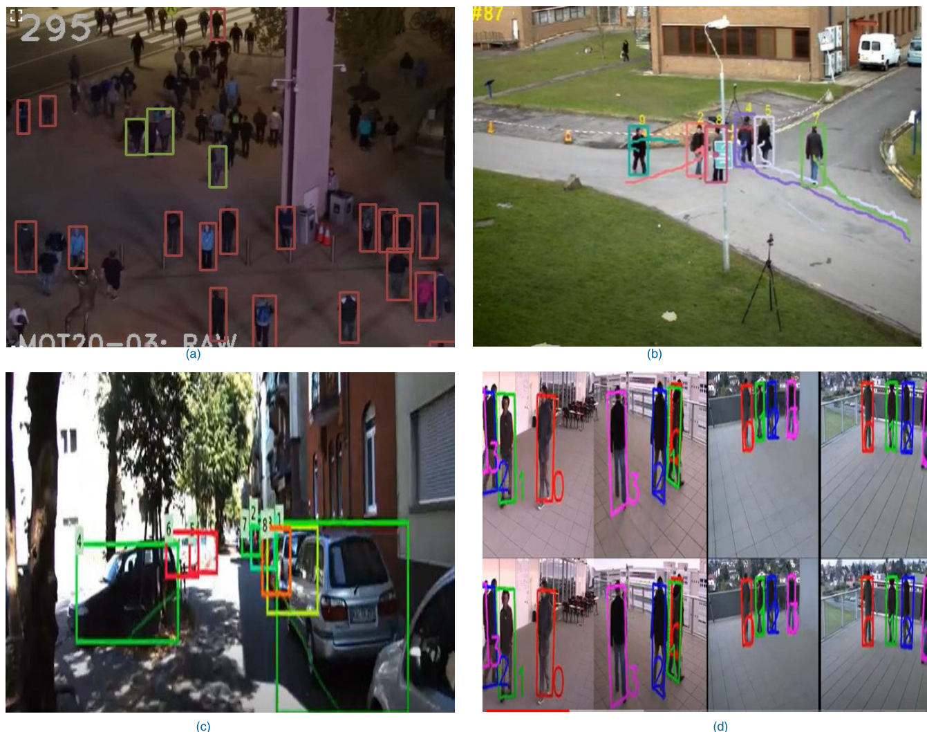
FIGURE 10. Illustration of the detections and feature learning with DLM-based online MOTs. (a). Insufficient detections (poor quality detections) in MOT2020 enter/exit stadium; (b) sufficient detection in PETS09-S211 sequence; (c) Real-time high-speed tracking with a mono-camera in KITTI and (d) multi-person tracking results, color features in deep learning.
