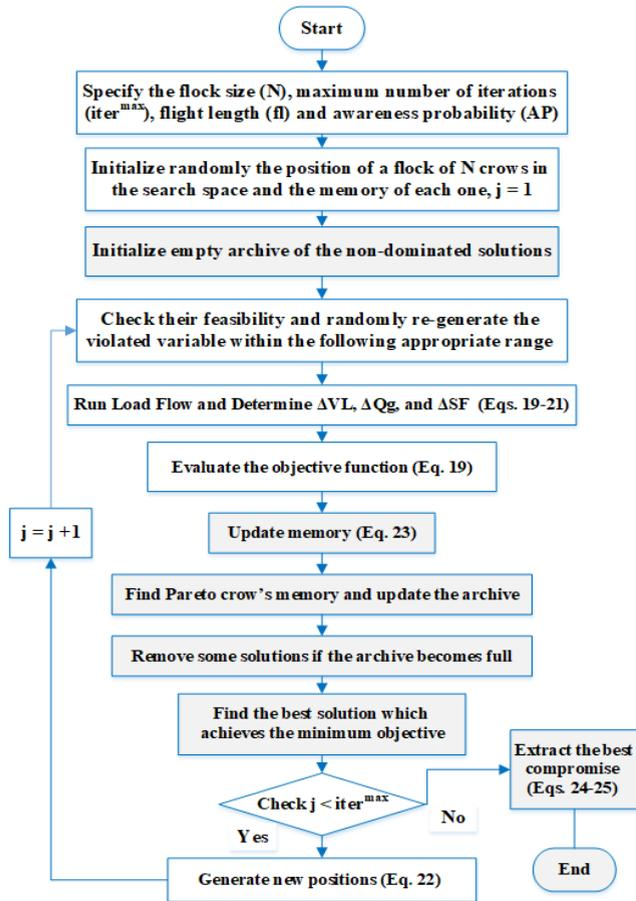
FIGURE 2. MCSO for handling the multi-objective EEPF.
