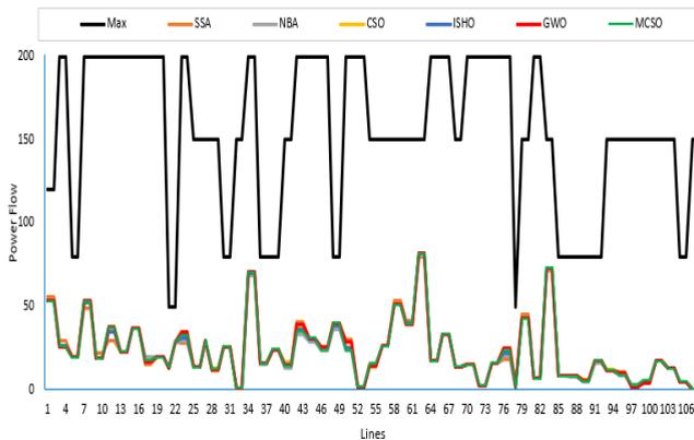
FIGURE 11. Power flow through the lines versus the maximum limits.
