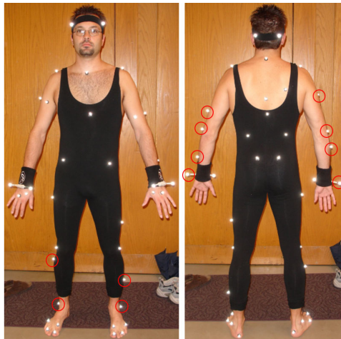
FIGURE 10. Marker position on the subject, the markers in the red circle is used in our test.
