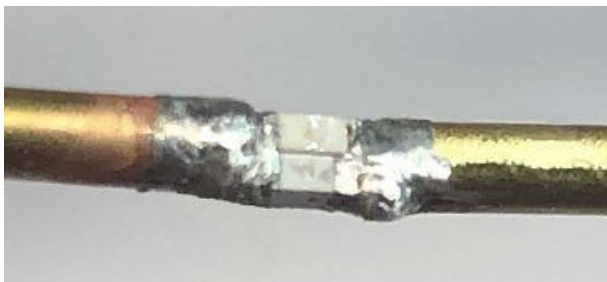
FIGURE 8. The capacitor and inductor of the 2 GHz trap are soldered together in parallel and to the inner and outer sections of the elements.
