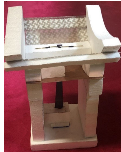
FIGURE 9. The complete fabricated reflector antenna prototype with the trapped dipole soldered to the MSL feed, FSS and rear reflectors, SMA connector and polystyrene mounts.
